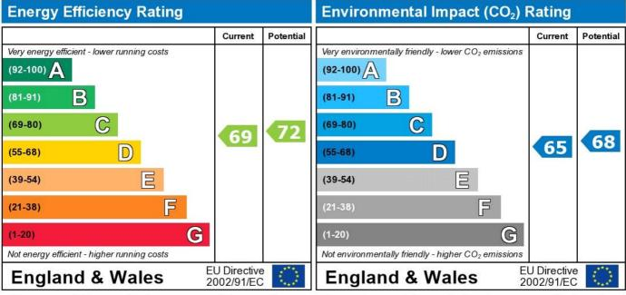
The energy efficiency rating is a measure of the overall efficiency of a home. The higher the rating the more energy efficient the home is and the lower the fuel bills will be. The environmental impact rating is a measure of a home's impact on the environment in terms of carbon dioxide (CO2)
